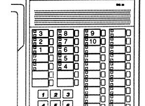
Figure 5B: Line numbering for Merlin 1030 Control Units.
